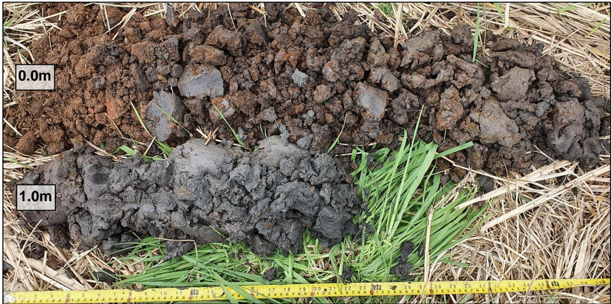
Figure 4: Bore 1 auger cuttings.
